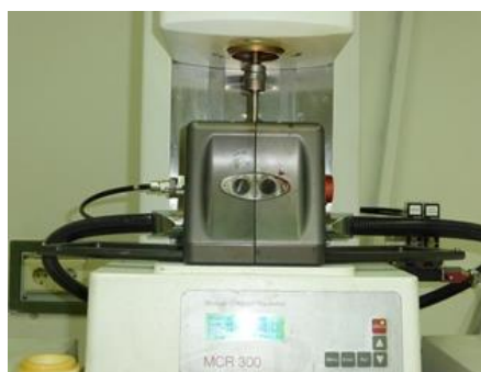
Figure3. shear reometer dynamic- model MCR300
